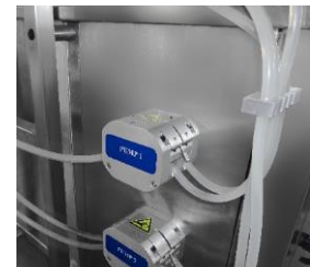
Figure 2 AccuFill head integrated in liquid filling machine
